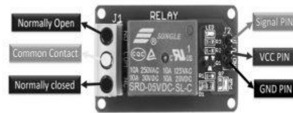
Fig 2.5 Pin Configuration of Relay Module
